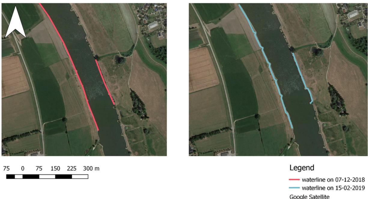
Figure 13 Waterline measurements by GPS \*07-12-18 missing the groynes extend
