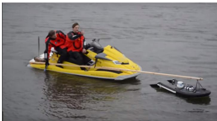
Figure 8 set-up: Jet-ski with the attached ADCP
